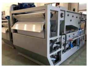
construction investment, etc, It is applicable to the solid-liquid separation of various suspended materials, especially the sludge dewatering process of large and medium-sized urban sewage plants and the dewatering of beneficiation paper mill and blast furnace waste residue.
